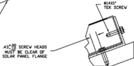
FIGURE 11 MOUNTING DETAIL FOR PEAK ROOF
